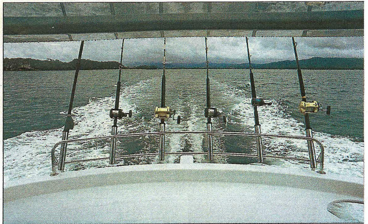
The rocket launcher accommodates up to six rods; six flush-mounted rod holders are fitted in the coamings and across the transom.
