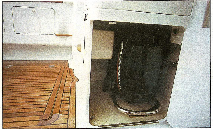
The outboard for Simply Red's tender is secured on a sliding cradle in its locker.
