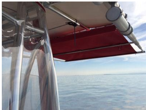
RTX INSTALLED ON T-TOP
